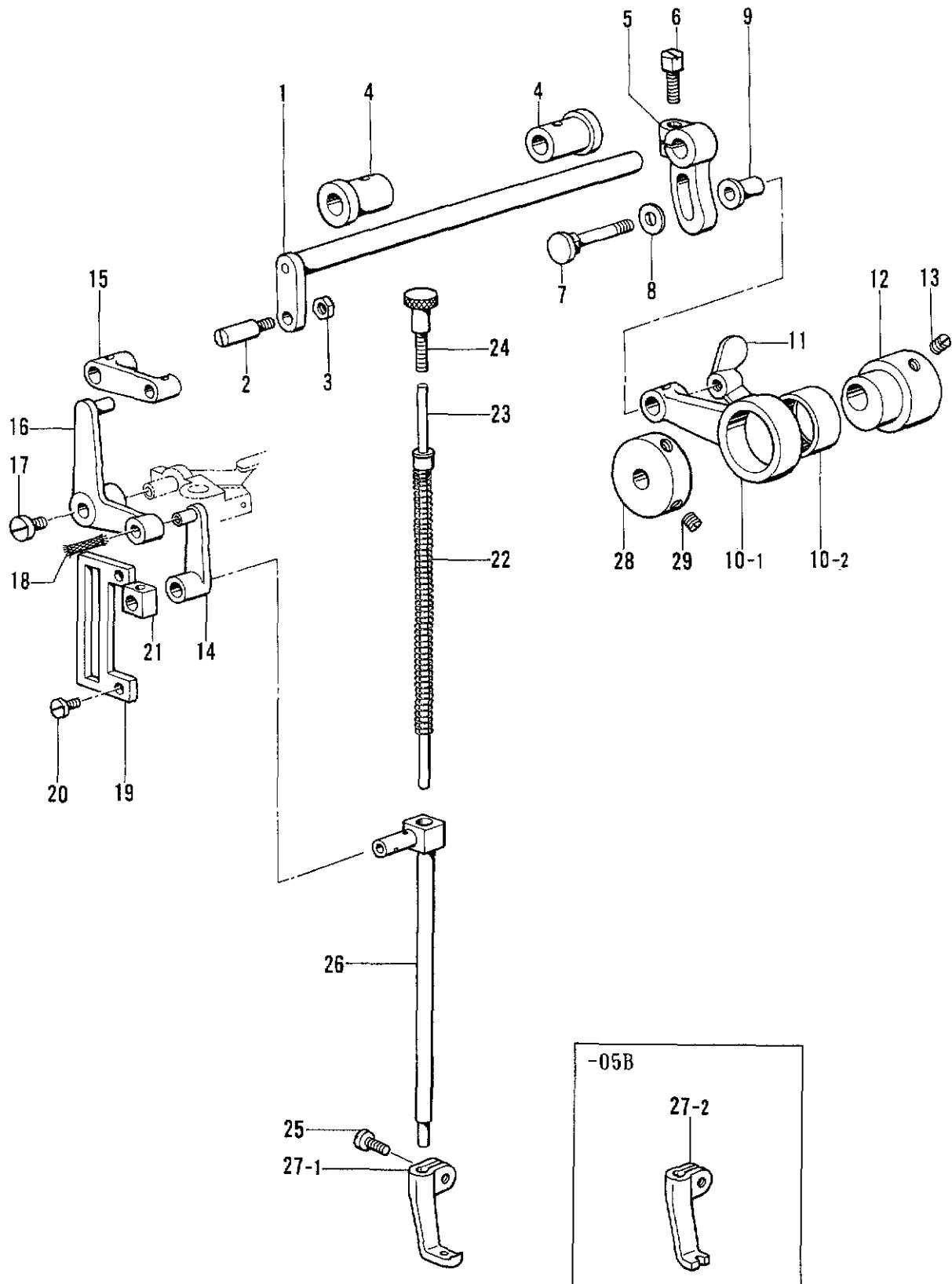
E. 上送り関係 /Upper feed mechanism/Obertransportvorrichtung/
