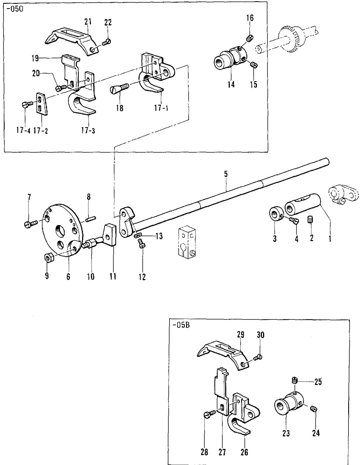
F. 送リ軸関係 /Feed shaft mechanism/Transport welle/
